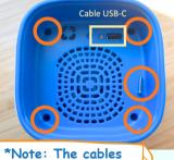
should not be squeezed by the plastic parts of the casing. Check inside the white casing for any areas that may press on the cables.
